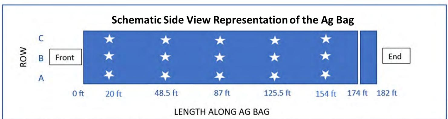
Row 'A' was 1 foot above grade, Row 'B' was ½ way up the bag and Row 'C' was on top of the bag. The stars represent the core points where outer cores were to 10 inch depth and inner cores were from 10 to 20 inch depth.
